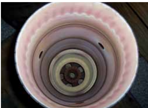
6B LEC-III™ liner at 14kFFH (Factored Firing Hours)
